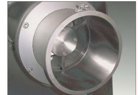
Extrusion screw to discharge the product in a form or shape, or directly to the next phase of processing.
