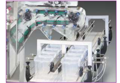
PLC controlled device for counting & filling lollipops into containers.
