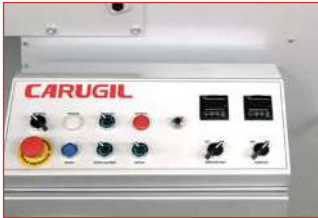
Control panel for monitoring the cooling process (humidity and temperature inside the cooling tunnel).
